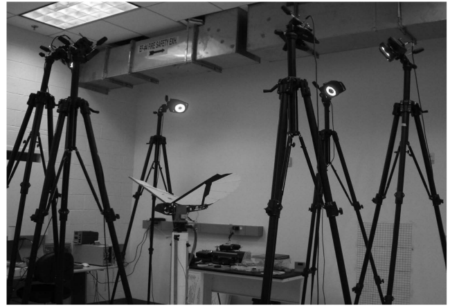
Fig. 1 Vicon® camera system used for the measurement of wing motion.
